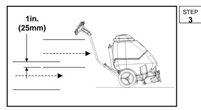
Push down on handle to raise vacuum shoe and brush before moving to the next cleaning pass. Overlap brush contact area a minimum of 1inch on the right (close cleaning) side of machine.
